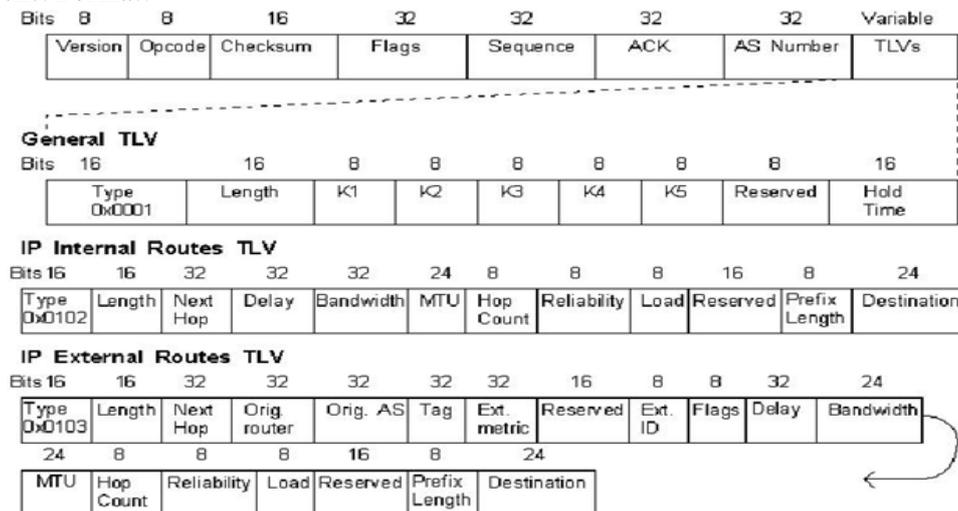
**Fig 2: EIGRP Packet format**
